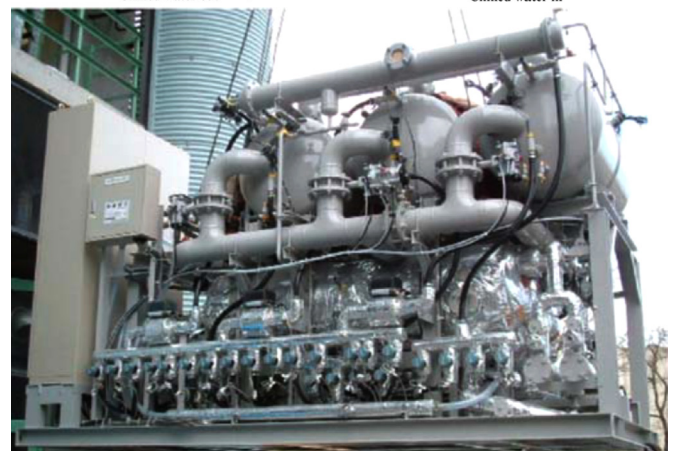
Fig. 2. A six-bed, silica gel–water, waste-heat driven ACS for building A/C applications designed by Saha et al. [43].
